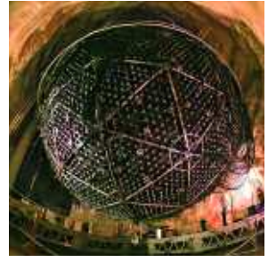
The SNO detector before the cavern was filled with water. SNO is nearly 2 km underground near Sudbury.
